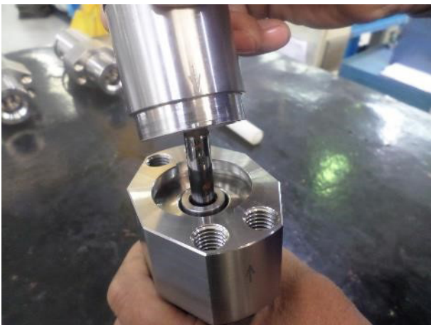
15. Insert the Frontal Stuffing-box
