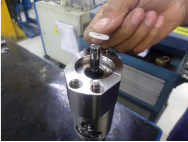
12. Insert the back ring (16). Compact it using a hammer and tube made of plastic
