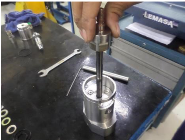
5. Insert the plunger in the stuffing box
