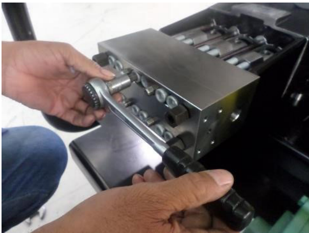
26. Torque screws M24x160 in cross mode by 3 steps: 50 / 100 / 140Nm.
