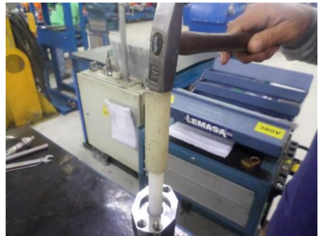
9. Compact it using a hammer and tube made of plastic
