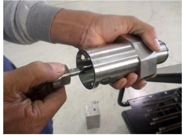
17. Remove the Plunger from the Stuffing Box
