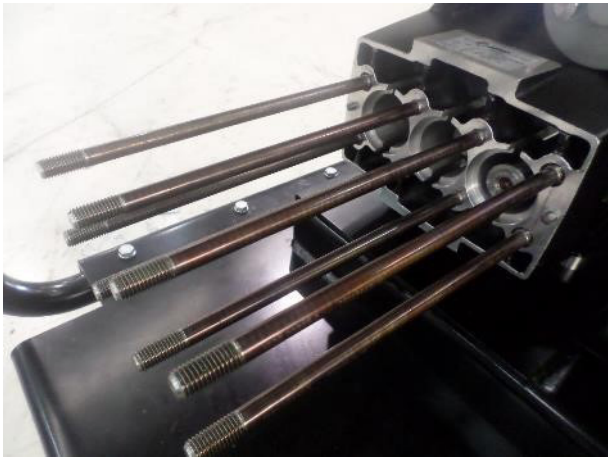
18. Screw the bolts in the crankcase
