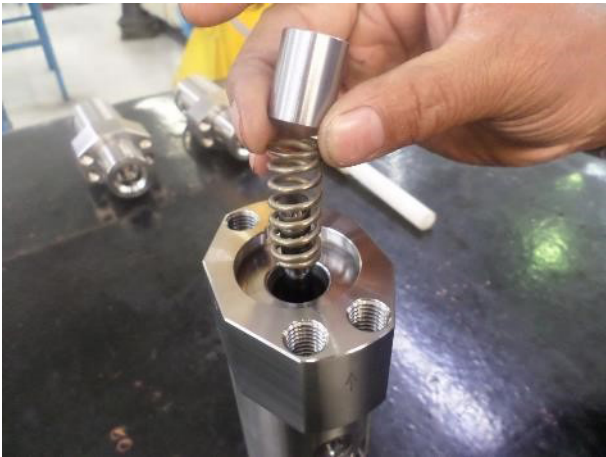
14. Insert the Spring (6) and Spring Support (5)
