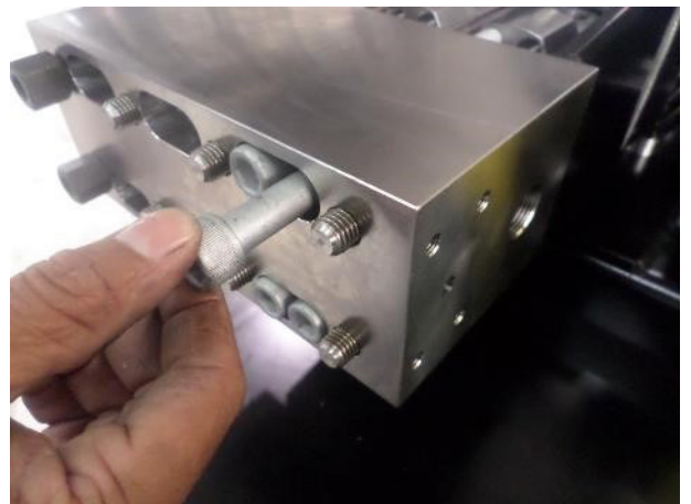
23. Insert the Screw M24x160 (without torque)
