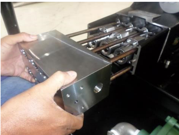
22. Insert the Fluid End and guide it using solid pin guide
