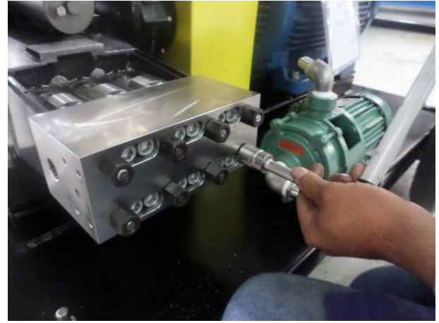
25. Torque it in cross mode by 3 steps: 30Nm / 60Nm / 100Nm.
