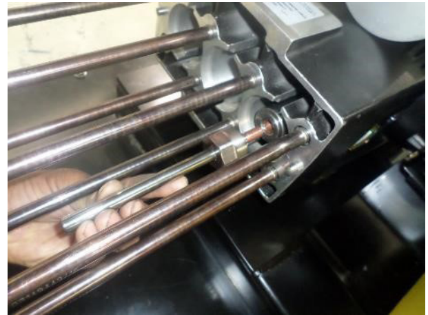
19. Screw the Plungers in the Plunger Guide
