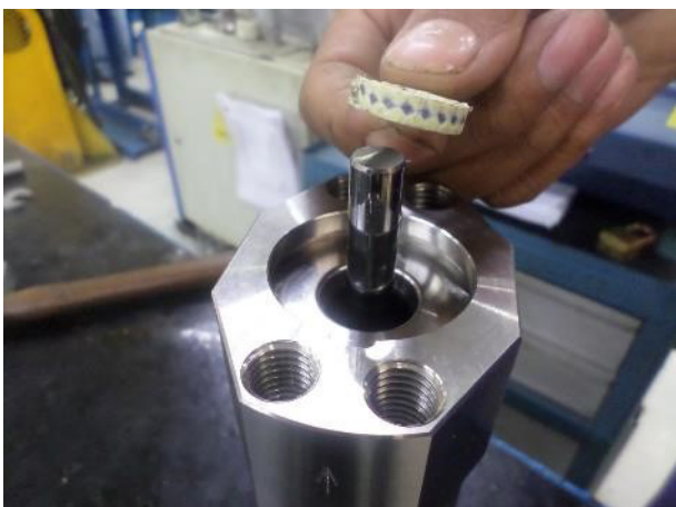
10. Insert the Gasket (15) and compact it using hammer and plastic tube.
