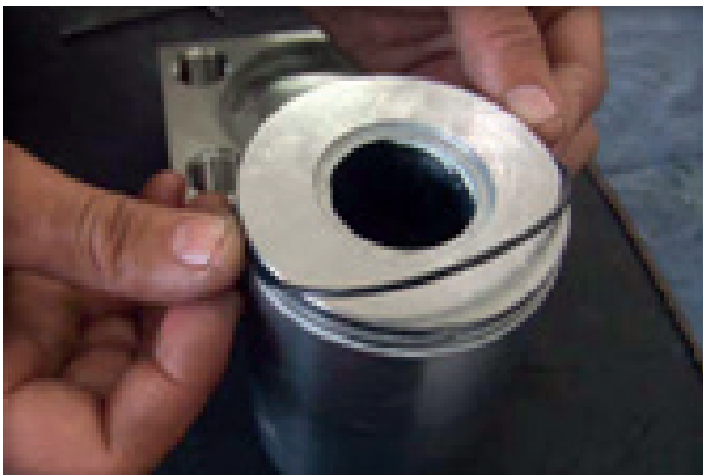
7° - Enter the O-Ring on tear shirt.
