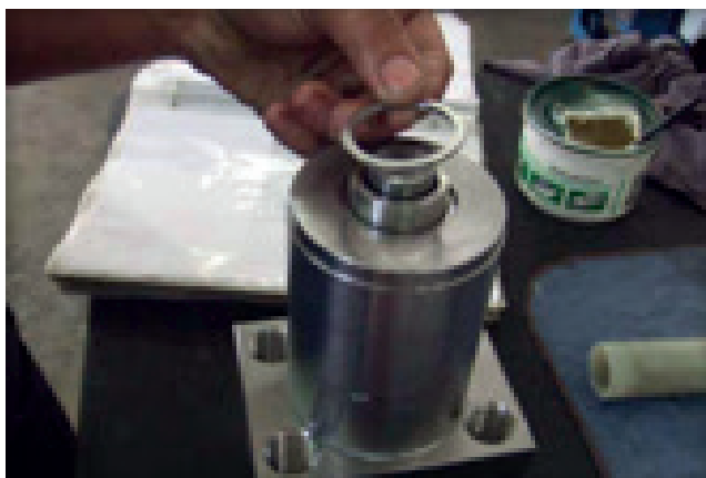
27° - Insert the upper metal seal.
