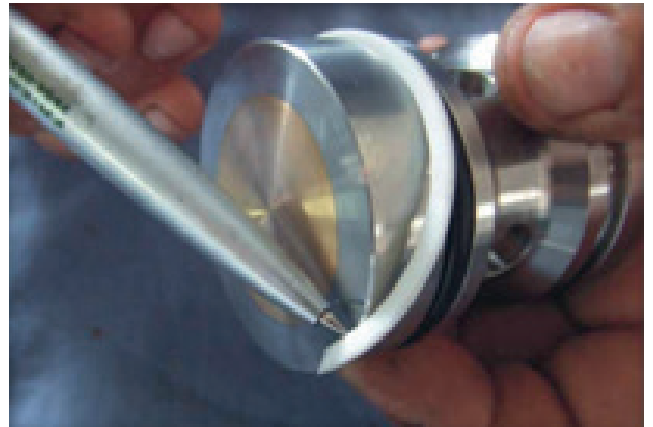
Put Bak ring, making sure that it is to the outside as well as the chamfer Bak Ring (indicated with the pen).
