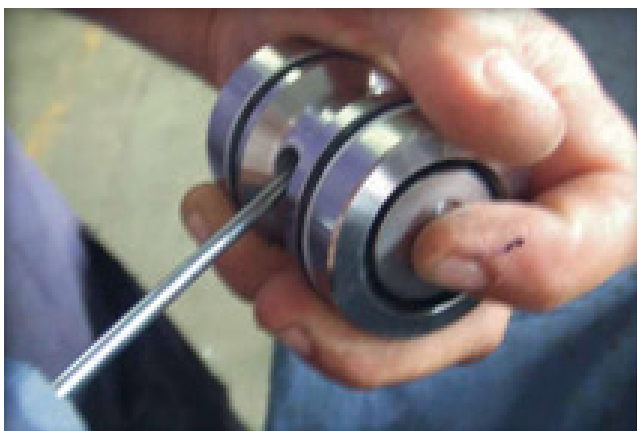
Attach the spring in Basket Cap, with the help of a key to attach it securely.
