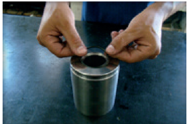
8° - When installing the shirt with the flange, the O-ring will be placed in recess.
