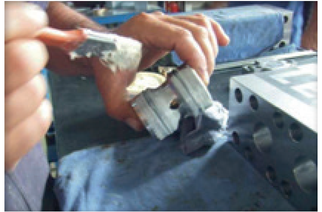
Pass desingripante grease also in Basket cap and place it on the head.
