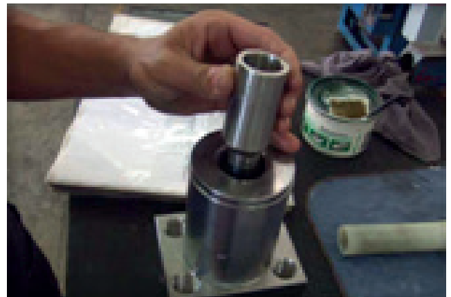
26° - Insert the bushing Support.
