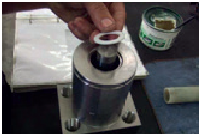
21° - Insert the other scraper ring.
