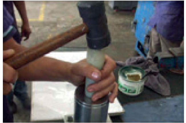
24° - Use a Nylon beater to pull the components.
