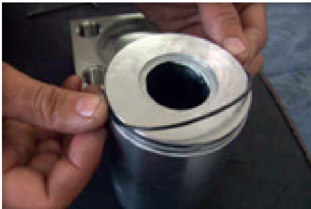
7° - Enter the O-Ring on tear shirt.
