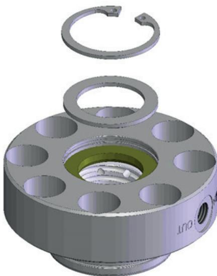
USE THE SPACER AND SEEGER TO FIX THE ASSEMBLED PARTS.
