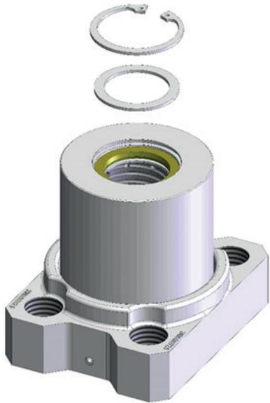
USE THE SPACER AND THE SEEGER TO FIX THE ASSEMBLED PARTS.
