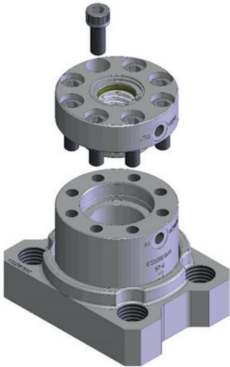
USE GREASE TYPE "ROCOL" ON THE SCREW THREADS M10 THE SUPPORT FLANGE WITH THE SLEEVE PERFORM THE TIGHTENING "X" WITH TORQUE TO 60Nm.
