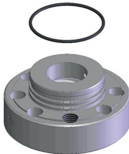
INSERT THE O-RING INTO THE SUPPORT FLANGE (USE GREASE TYPE "ROCOL" TO IMPROVE THE SEALING).
