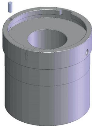
INSERT THE GUIDE PIN INTO THE SLEEVE.
