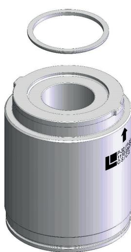
INSERT THE LOWER METAL RING WITH THE RADIUS FACING DOWNWARDS.
