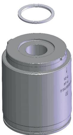
INSERT THE LOWER METAL RING WITH THE RADIUS FACING DOWNWARDS.
