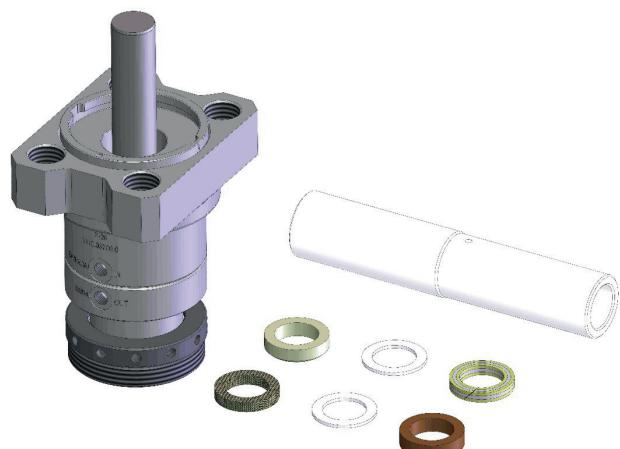
ARRANGE THE SEALING KIT ON THE WORK BENCH.
