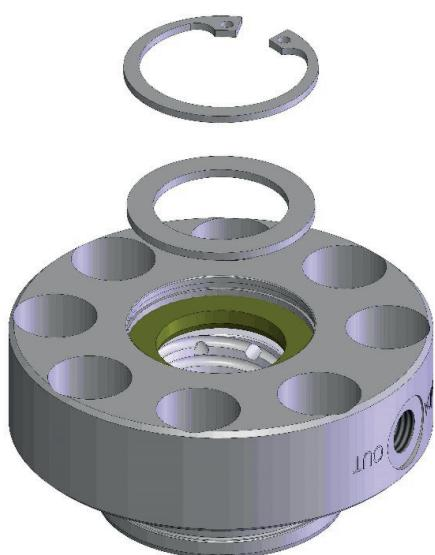
INSERT THE SPACER AND THE SEEGER RING TO FIX THE ASSEMBLED PARTS.
