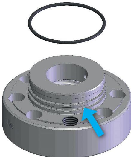
INSERT THE O-RING INTO THE SUPPORT FLANGE SEAT (SEE THE PICTURE).
