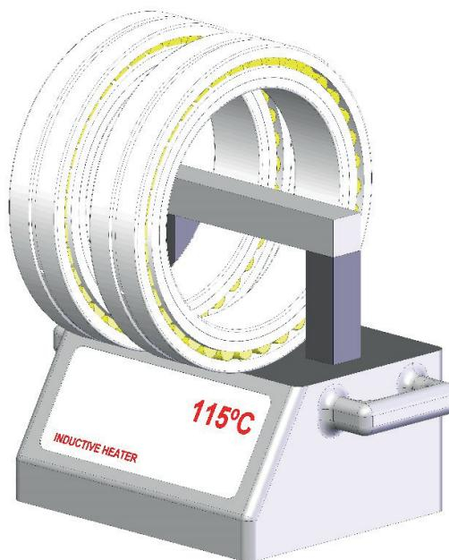
HEAT THE PAIR OF CRANKSHAFT BEARINGS AT 115°C FOR 10 MINUTES.
