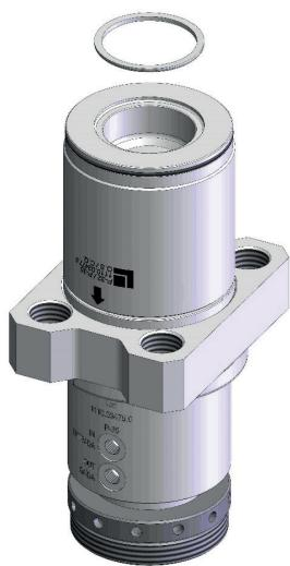
INSERT THE UPPER METAL RING WITH THE RADIUS FACING DOWNWARDS.
