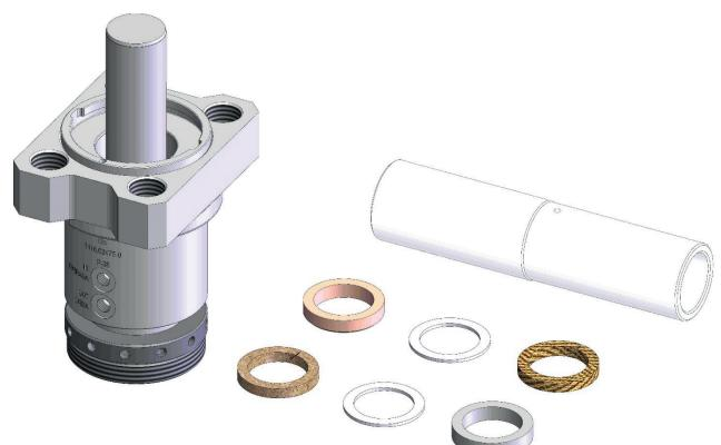
ARRANGE THE SEALING KIT ON THE WORK BENCH.
