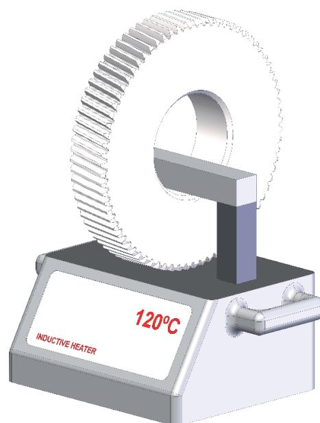
HEAT THE CROWN GEAR AT 120°C FOR 10 MINUTES.
