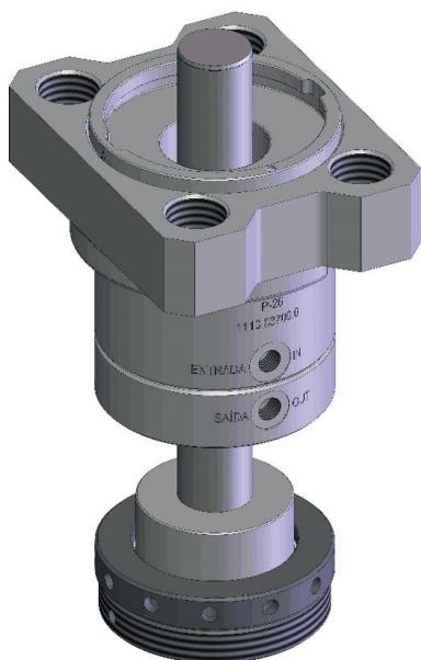
INSERT THE SLEEVE ASSEMBLED WITH THE FLANGE INTO THE PLUNGER UNTIL IT REACHES THE PLUNGER HEAD.
